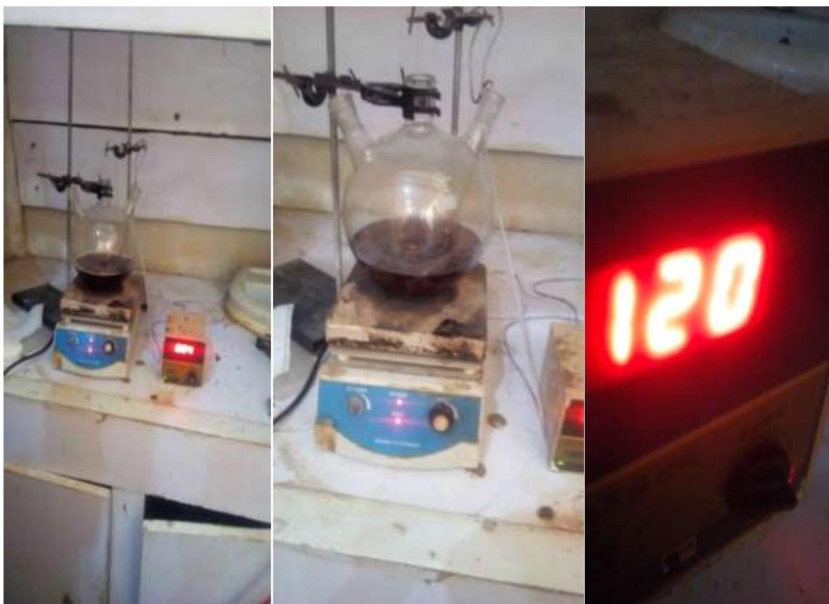
Figure 2: Jatropha and castor oil TMP esters biolubricant synthesis experimental setup
